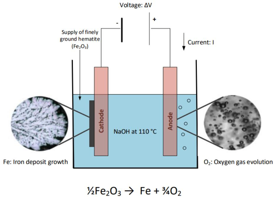
**Figure 16. Basic schematic of iron ore electrolysis**
