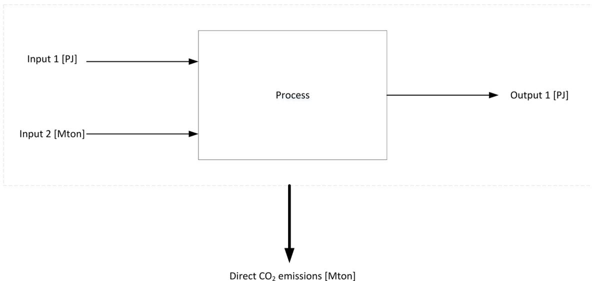
**Figure 7. Schematic of CO<sub>2</sub> emission calculation example**
