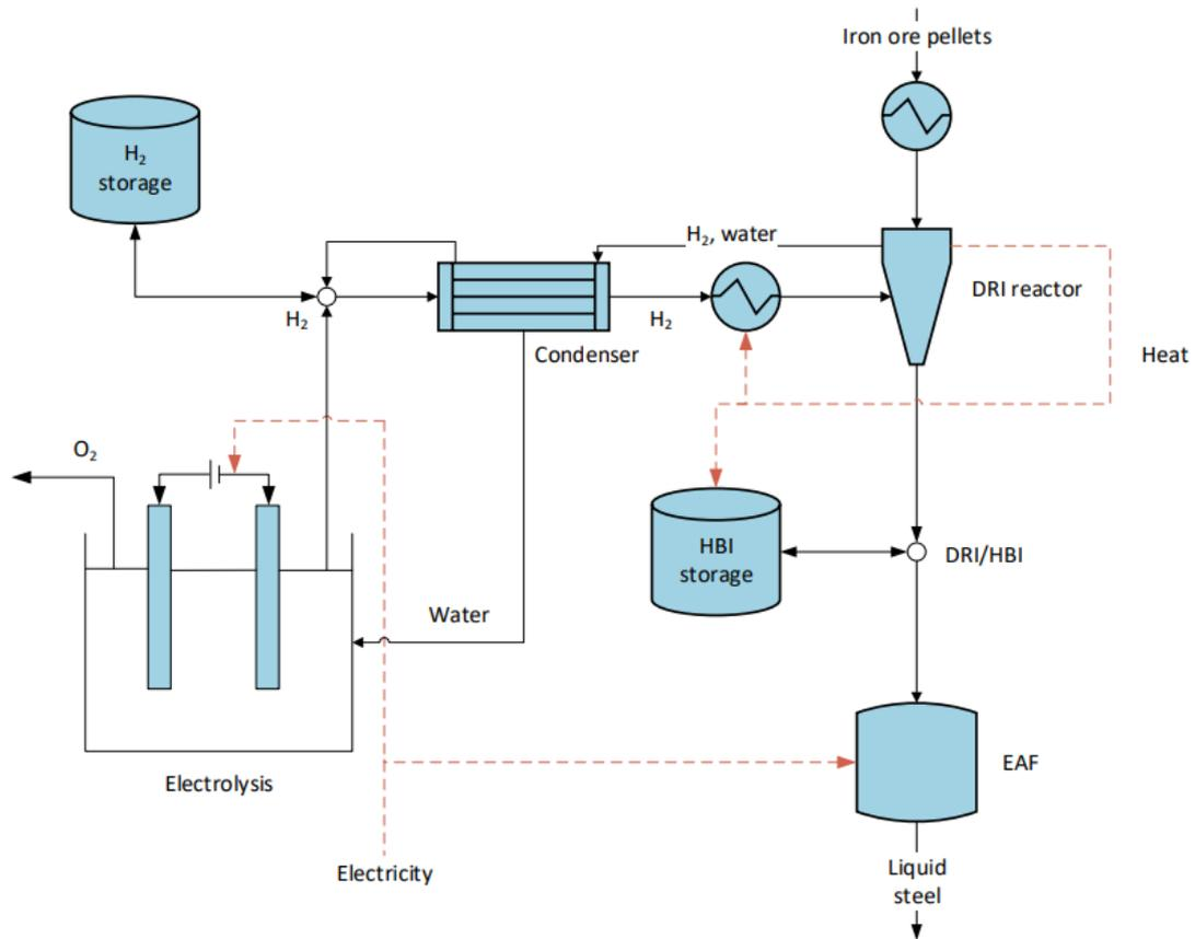
**Figure 15. Example schematic of hydrogen-based direct reduction**
