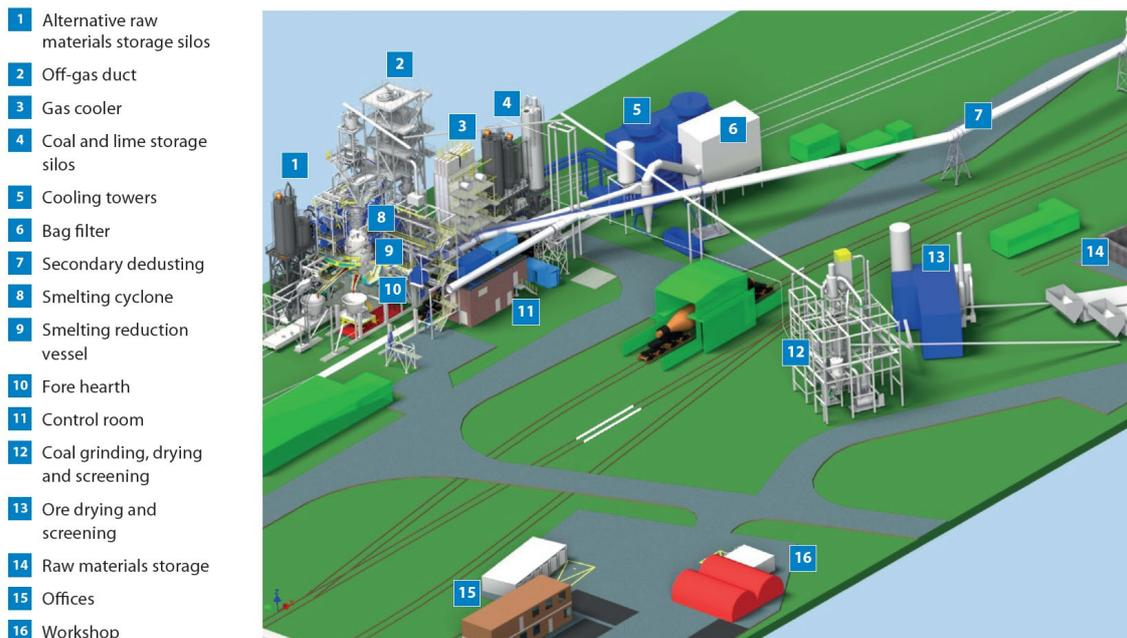
**Figure 13. Layout of HISarna pilot plant at TSIJ**
