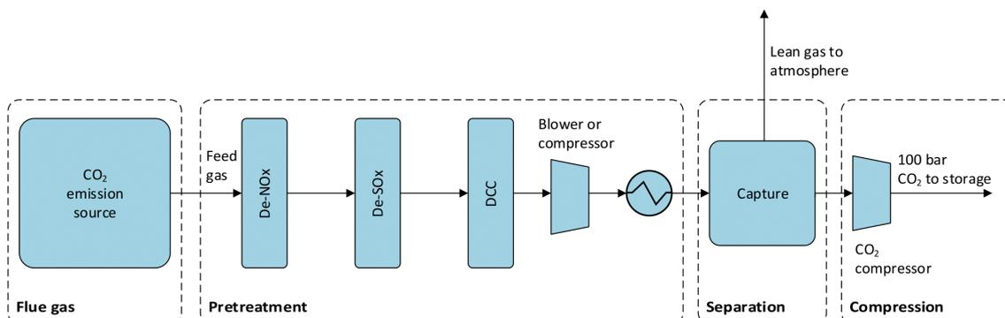
**Figure 29. Scope of CO<sub>2</sub> capture process**
