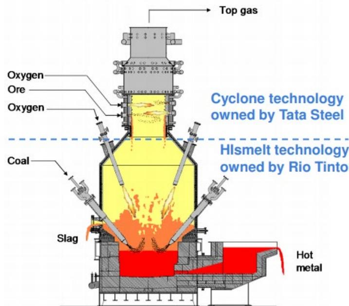
**Figure 12. Simplified schematic of the HIsarna process with CCS**
