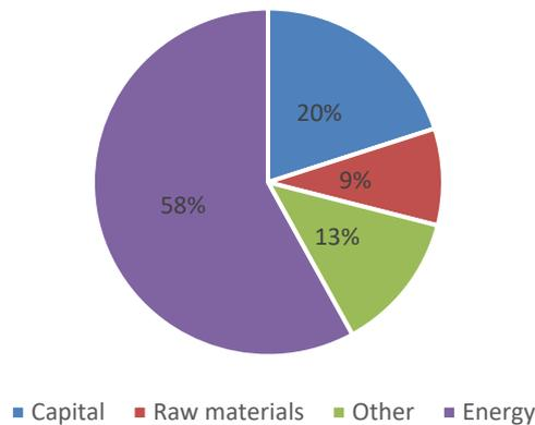
**Figure 33. Cost breakdown for CO<sub>2</sub> capture (MEA solvent) at a conventional steel mill power plant**
