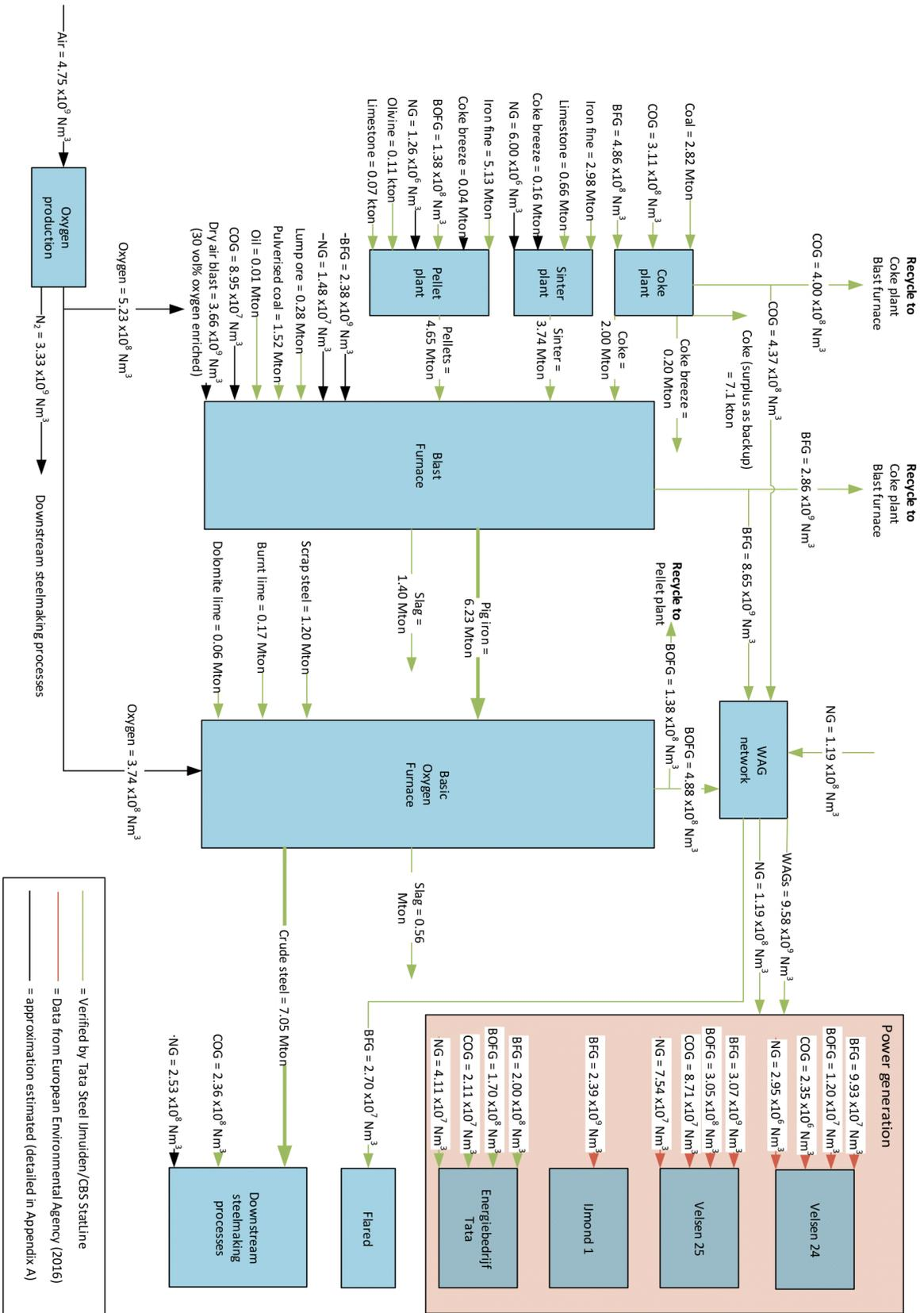
Figure 4. Annual material flow overview of the steelmaking process.
