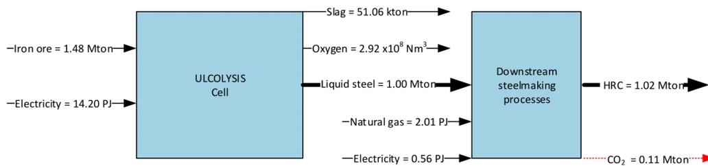
**Figure 28. Flowsheet of the ULCOLYSIS steelmaking route**
