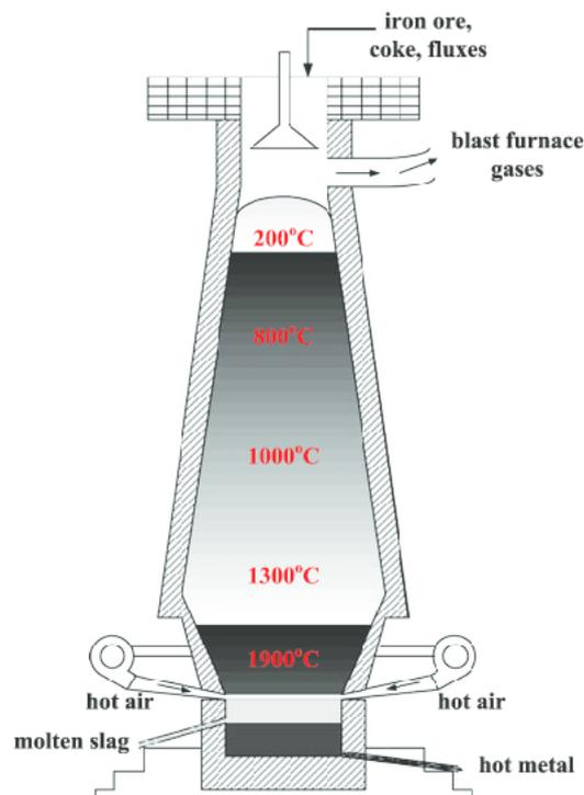
**Figure 3. Schematic diagram of the blast furnace process**
