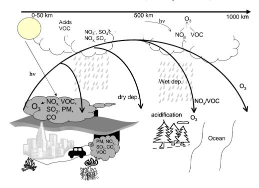
Figure 6.1 Interactions between pollutants, with the short-distance (urban air pollution), and long-distance (acidification) impacts indicated. The influence of solar radiation, some transforming processes, and deposition processes are also depicted
