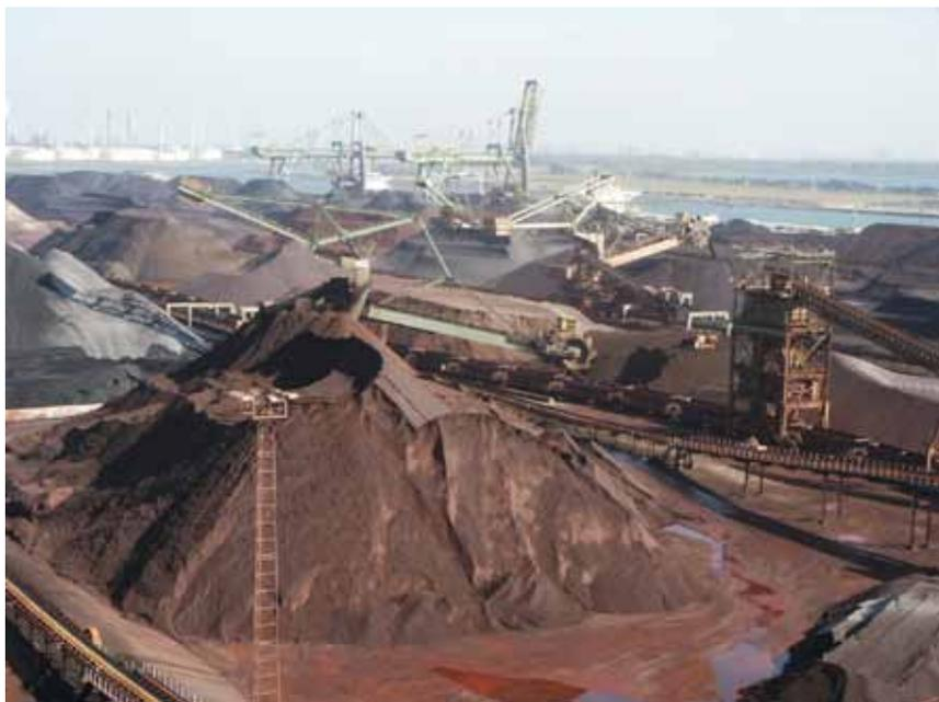
Material handling (loading, unloading, stockpiling, blending, transporting) is a potential source of mineral PM<sub>10</sub>.
