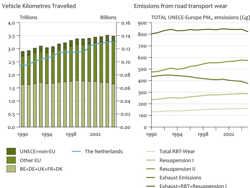
Trend in average vehicle distances travelled (left panel), and in calculated PM<sub>10</sub> emissions from road transport: exhaust emissions, road wear, tyre wear, brake wear, and approximated resuspension of dust due to traffic (right panel).
