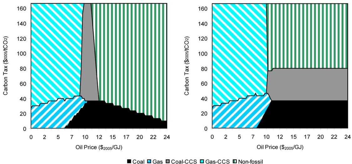
Figure 5.4 Cheapest electricity production options with different oil/gas/coal prices and carbon tax levels
