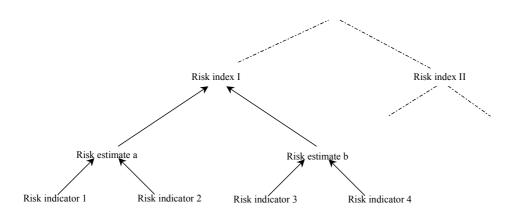
*Figure 13 – Aggregation procedure for composite risk estimates.*
