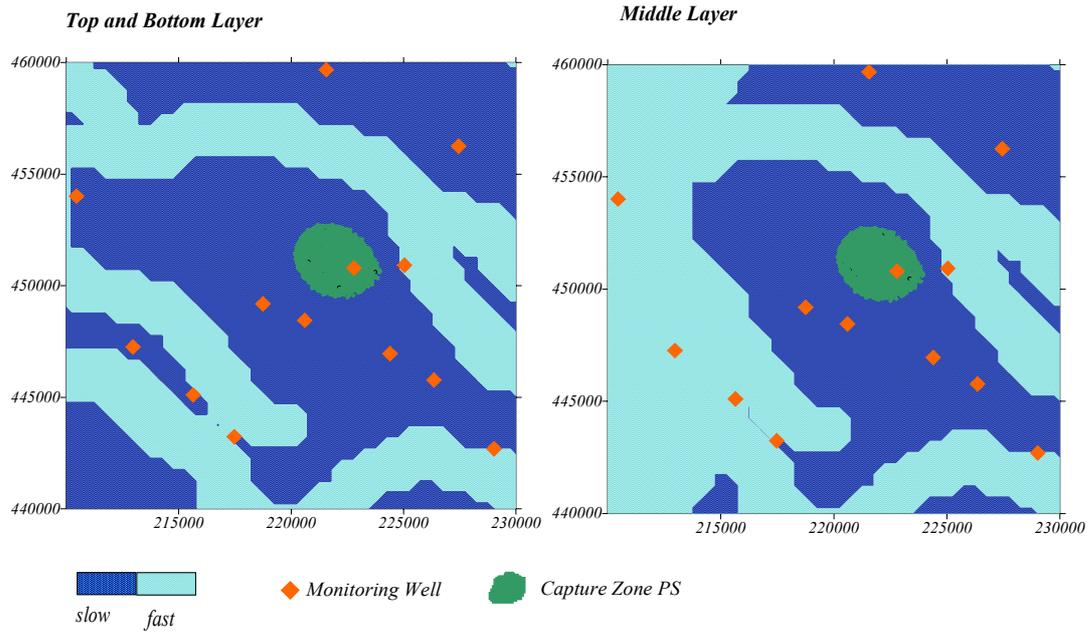
Figure 21. Location of monitoring wells and capture zone for pumping station **Klooster** with zonation of denitrification parameter.
