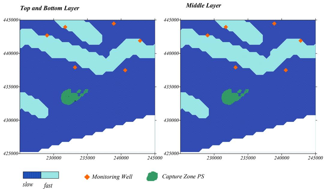
Figure 22. Location of monitoring wells and capture zone for pumping station **Dinxperlo** with zonation of denitrification parameter.
