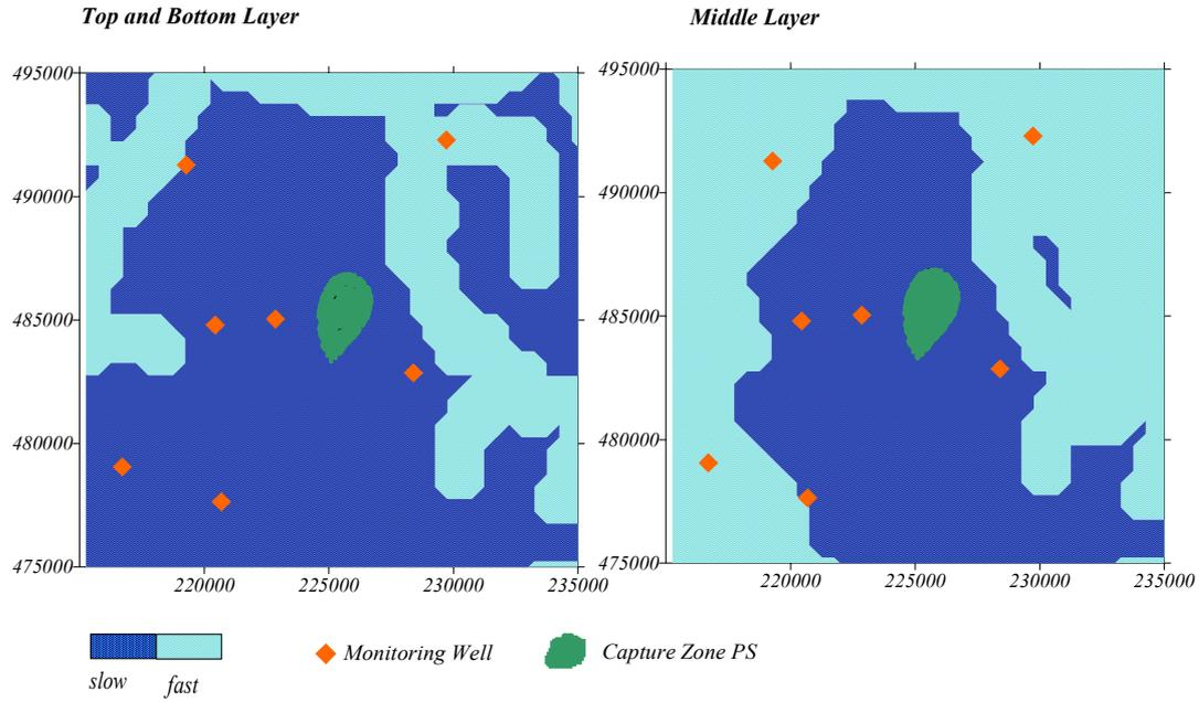
Figure 23. Location of monitoring wells and capture zone for pumping station *Nijverdal* with zonation of denitrification parameter.
