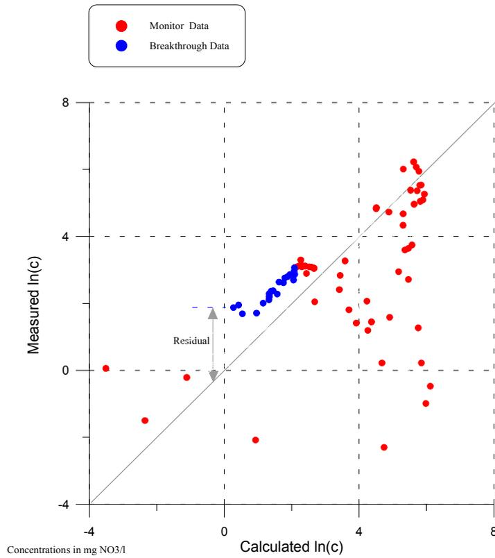
Figure 32. Measured data versus model results for the pumping station **Putten**.
