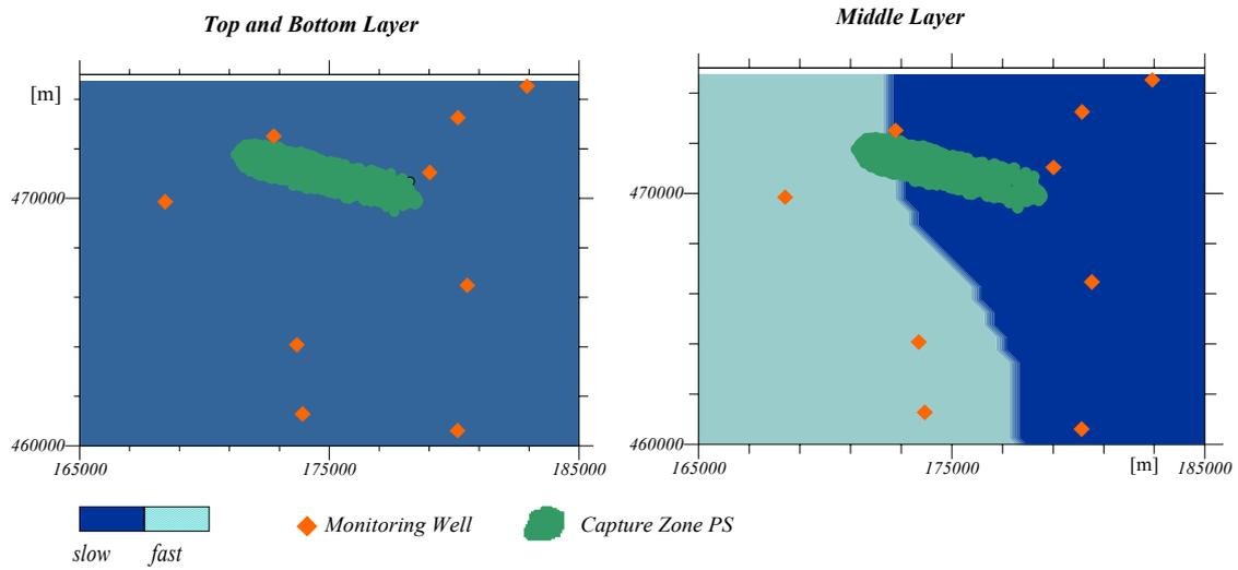
Figure 25. Location of monitoring wells and capture zone for pumping station **Putten** with zonation of denitrification parameter.
