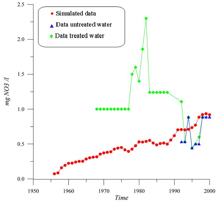
Figure 33. Comparison of simulated breakthrough curve with measured data for the pumping station Coevorden.
