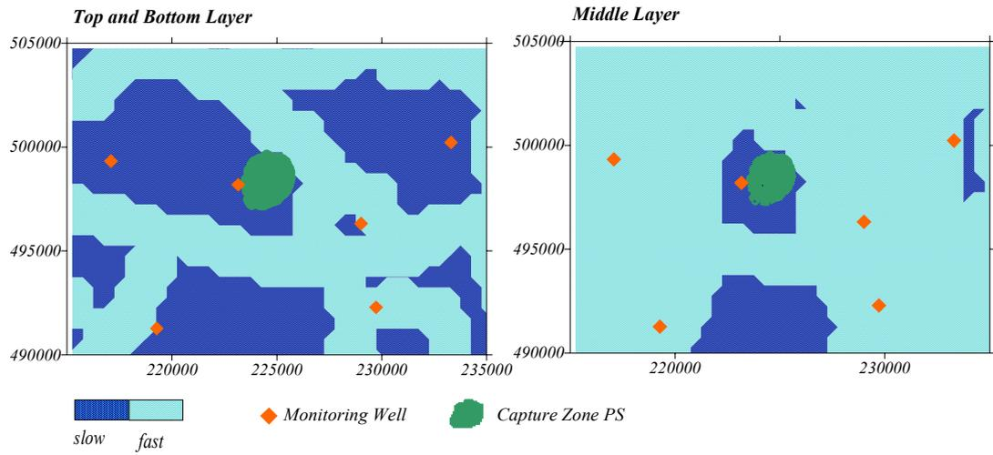
Figure 19. Location of monitoring wells and capture zone for pumping station **Archemerberg** with zonation of denitrification parameter as background.
