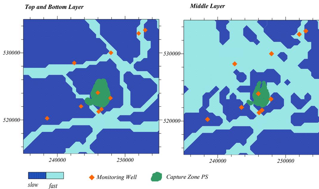
Figure 26. Location of monitoring wells and capture zone for pumping station **Coevorden** with zonation of denitrification parameter.
