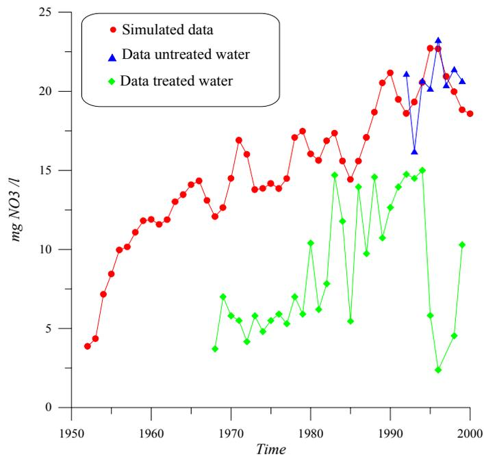
Figure 27. Comparison of simulated breakthrough curve with measured data for the pumping station **Herikerberg**.
