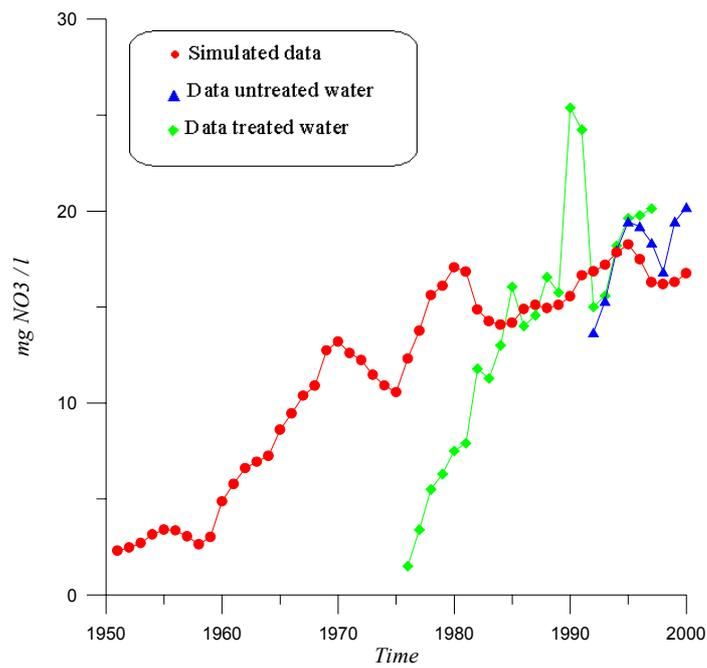
Figure 29. Comparison of simulated breakthrough curve with measured data for the pumping station *Archemerberg*.
