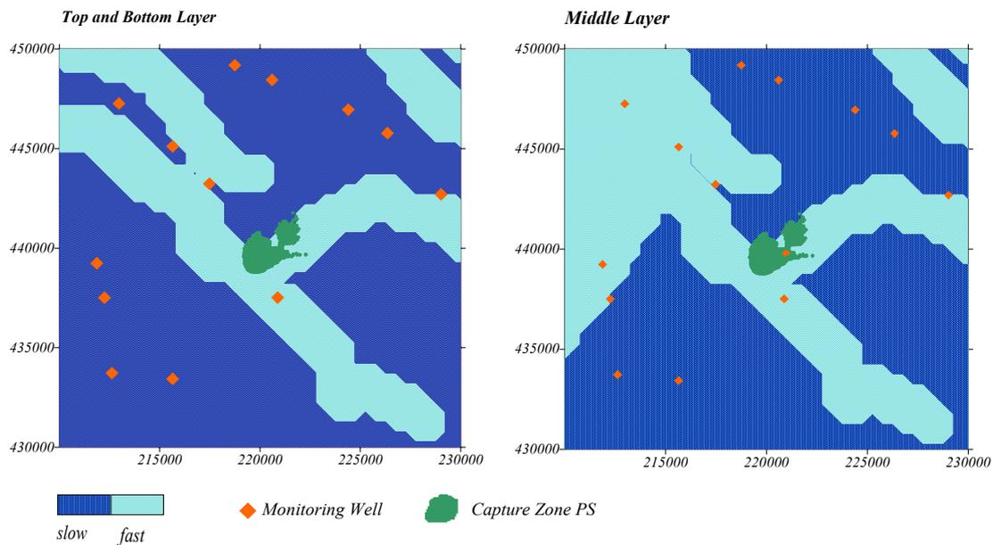
Figure 18. Location of monitoring wells and capture zone for pumping station **De Pol** with zonation of denitrification parameter as background.
