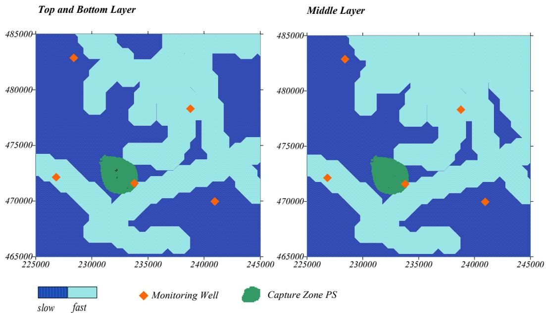
Figure 20. Location of monitoring wells and capture zone for pumping station **Herikerberg** with zonation of denitrification parameter as background.
