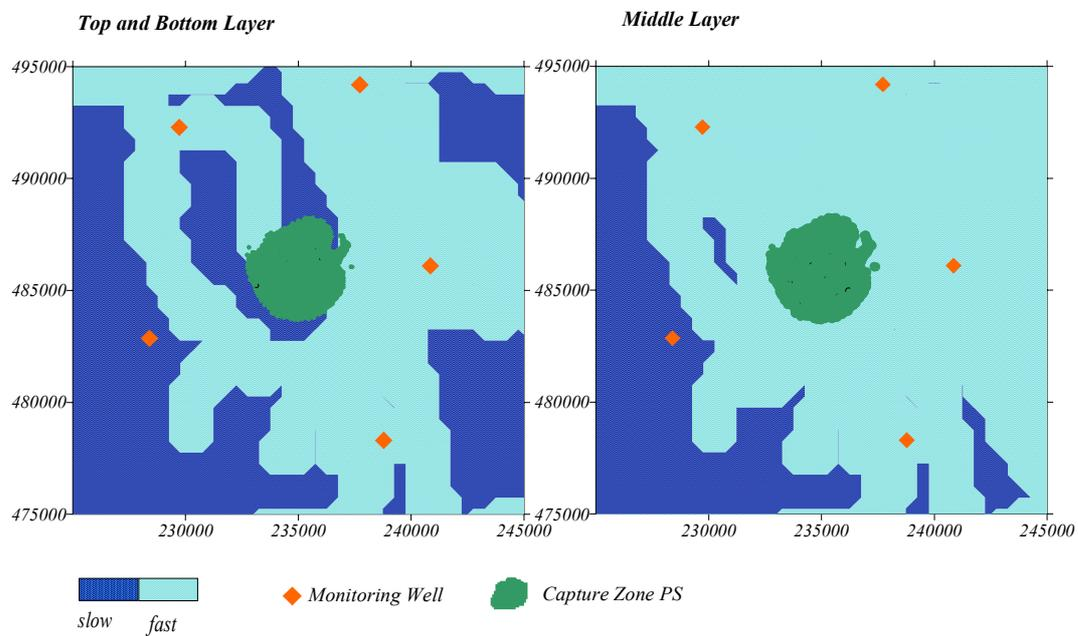
Figure 24. Location of monitoring wells and capture zone for pumping station *Wierden* with zonation of denitrification parameter.
