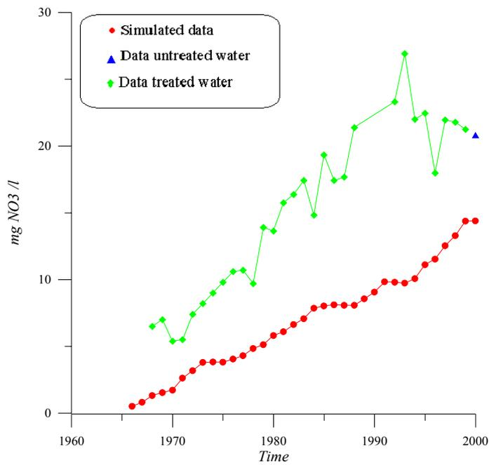
Figure 31. Comparison of simulated breakthrough curve with measured data for the pumping station **Putten**.
