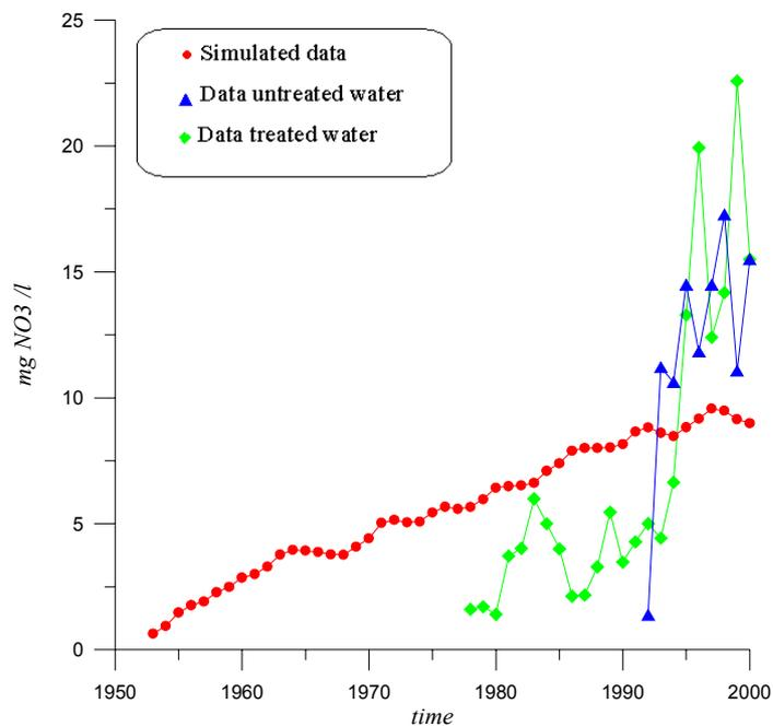
Figure 28. Comparison of simulated breakthrough curve with measured data for the pumping station **Dinxperlo**.
