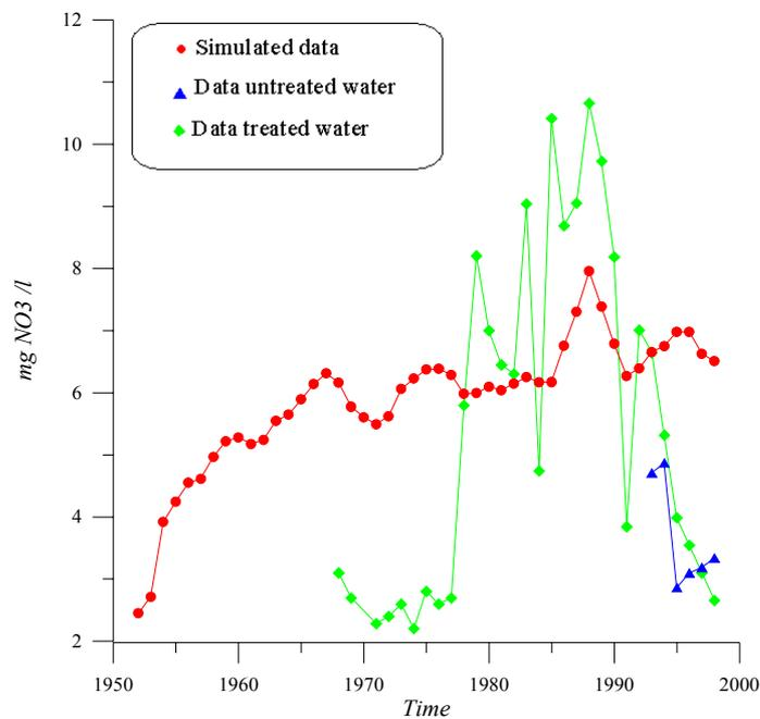
Figure 30. Comparison of simulated breakthrough curve with measured data for the pumping station *De Pol*.
