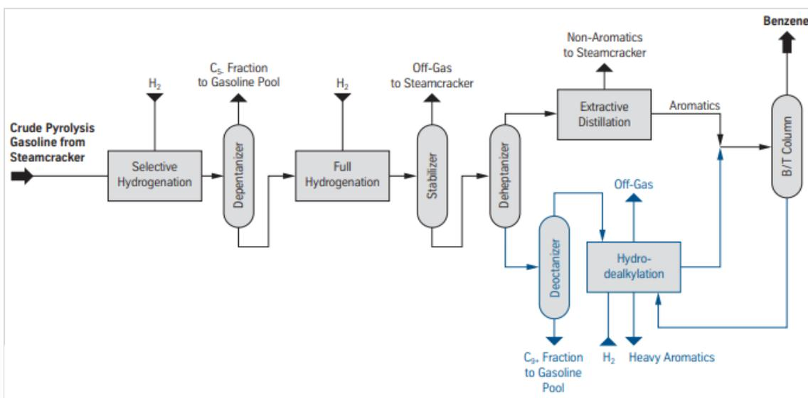
**Figure 2.3 Benzene extraction from crude pyrolysis gasoline of the steam cracker (Thyssen-Krupp, 2014)**
