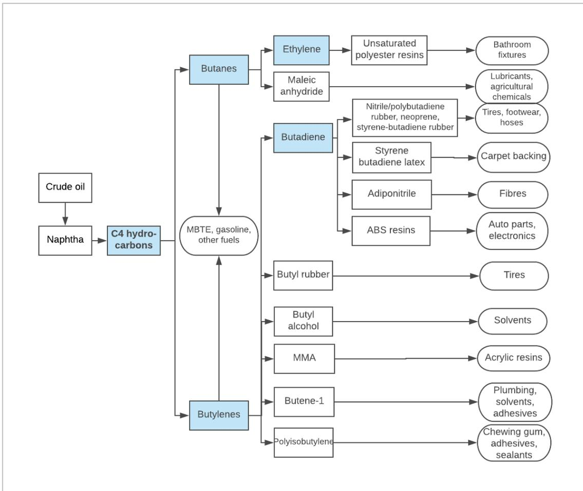
**Figure 3.5 Production chain for C4 hydrocarbons, blue boxes indicate chemicals produced at Shell Moerdijk adapted from (ACC, 2017)**
