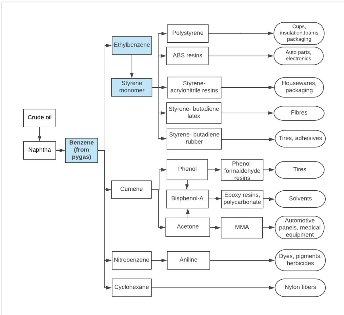
**Figure 3.6. Production chain for benzene, blue boxes indicate chemicals produced at Shell Moerdijk (adapted from ACC, 2017)**
