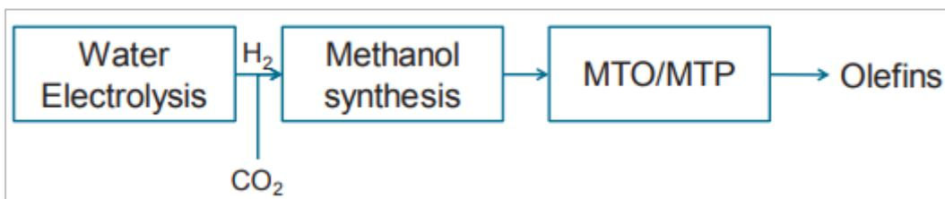
**Figure 4.3 Ethylene/propylene production from methanol (Dechema, 2017)**
