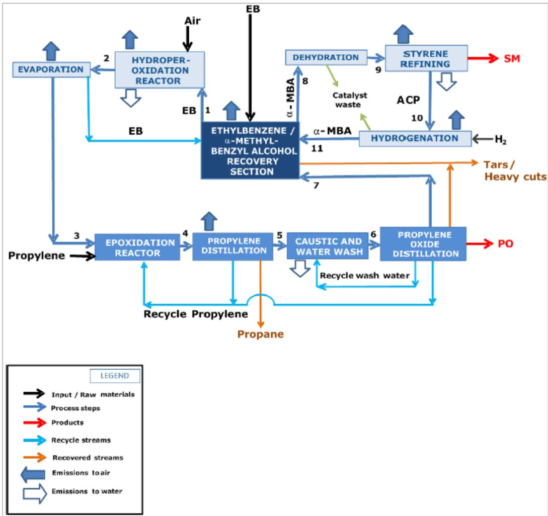
Figure 2.7 Flow diagram of EB peroxidation process to co-produce SM and PO, numbers represent steps of the reaction (Falcke, et al., 2017)
