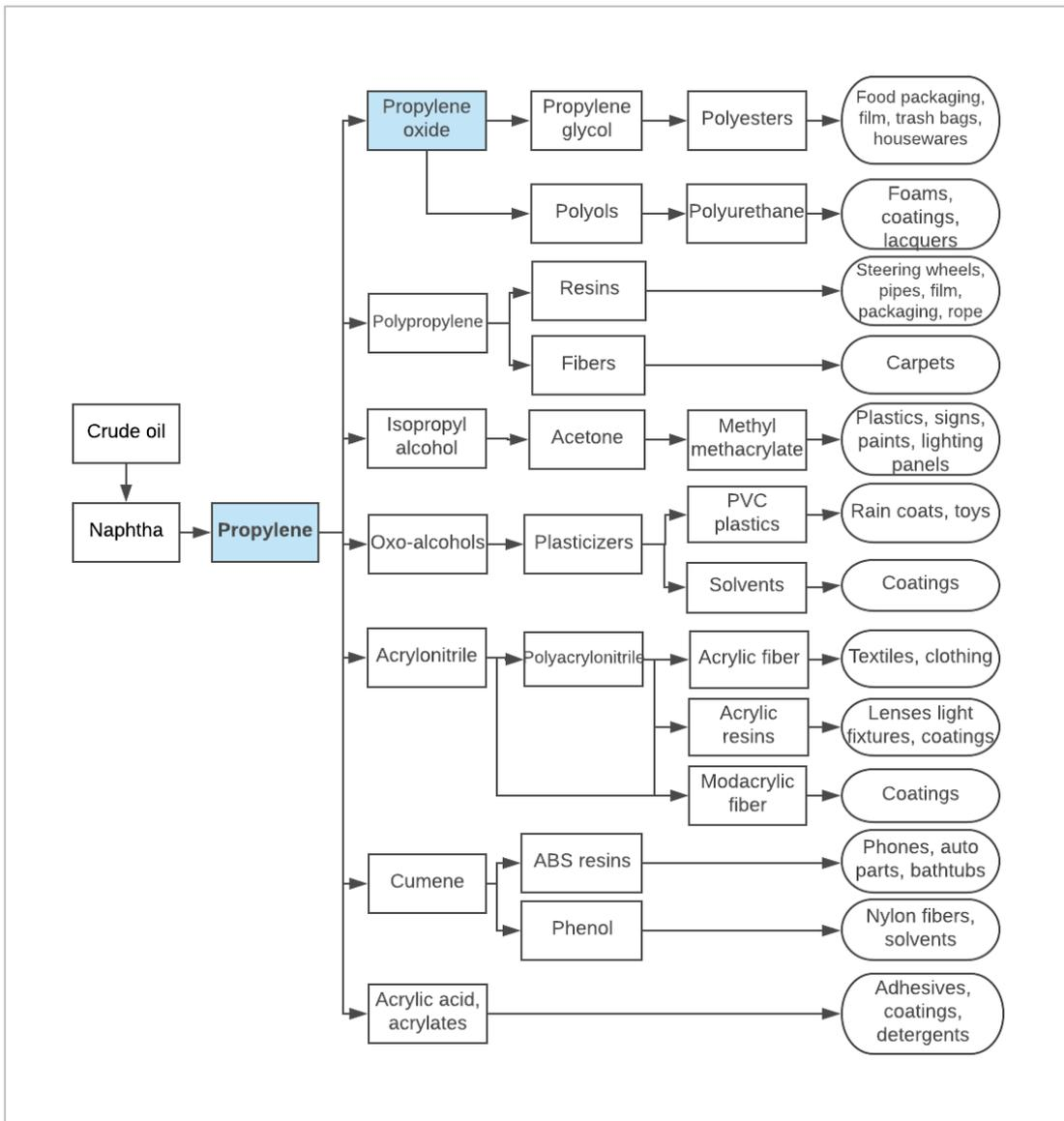
**Figure 3.4 Production chain for propylene, blue boxes indicate chemicals produced at Shell Moerdijk (adapted from ACC, 2017)**
