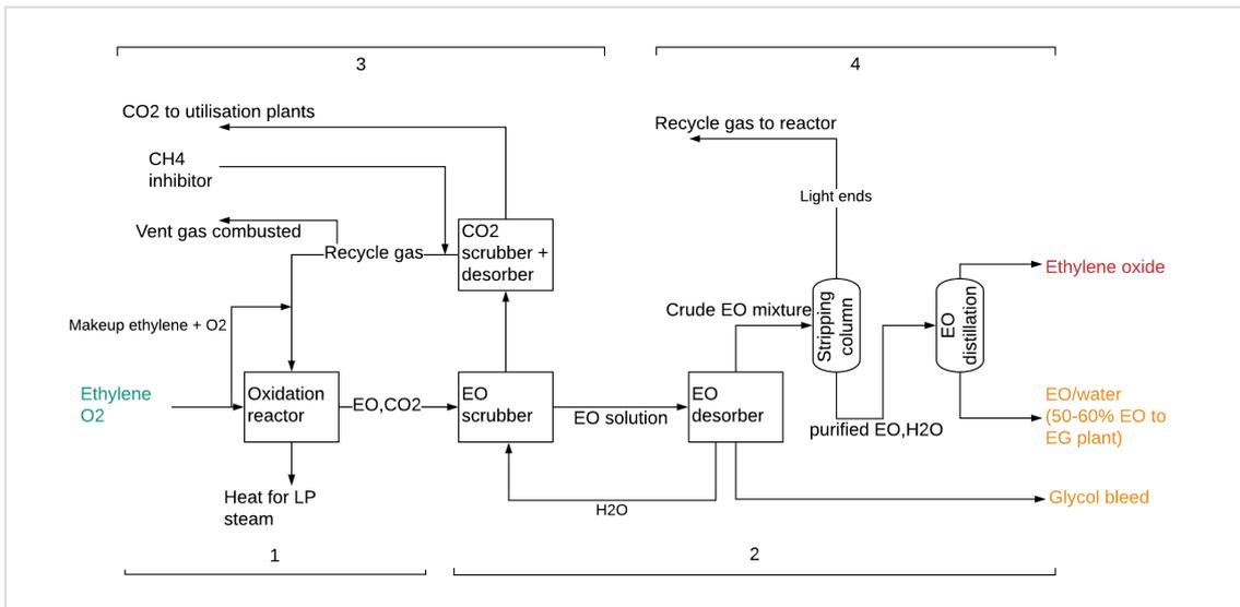
**Figure 2.4 EO production process from ethylene**
