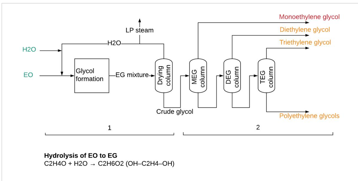
**Figure 2.5 MEG, DEG, TEG, and polyethylene glycols production from ethylene oxide**
