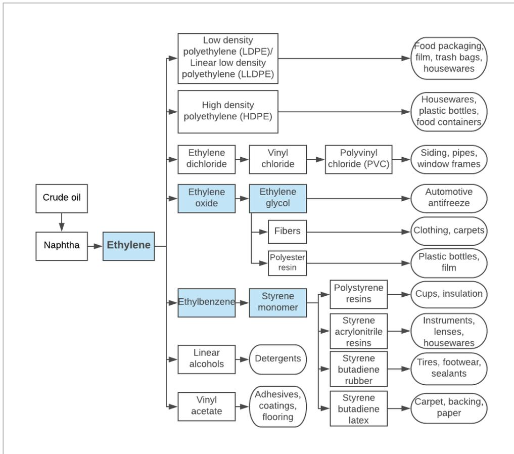
**Figure 3.3 Production chain for ethylene, blue boxes indicate chemicals produced at Shell Moerdijk (adapted from ACC, 2017)**
