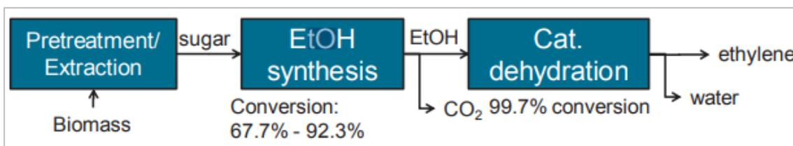
**Figure 4.2 Ethylene production from bioethanol (Dechema, 2017).**
