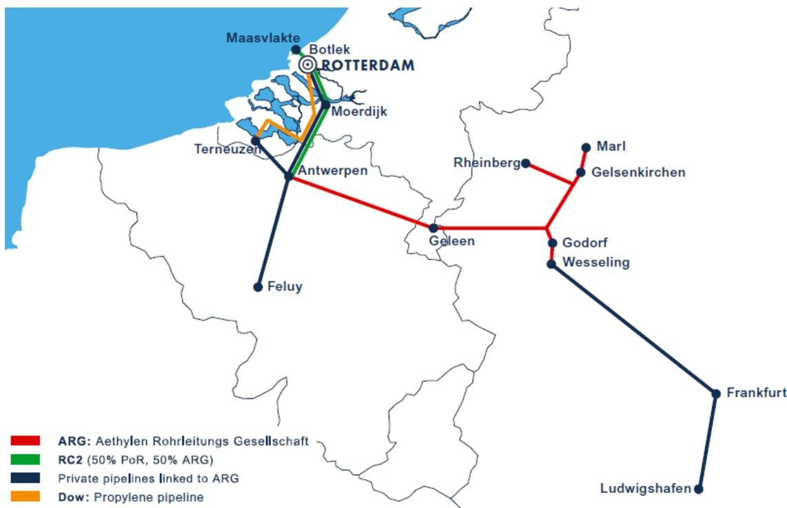
**Figure 1.2 Ethylene and propylene pipelines in the ARRR cluster (Port of Rotterdam, 2010)**
