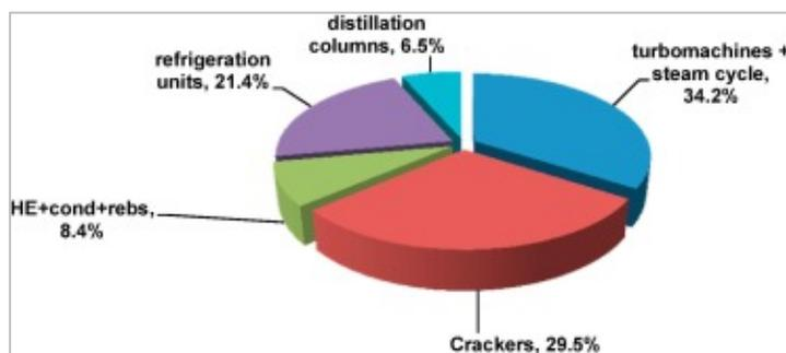
**Figure 2.8 BEC for plant components, as a percentage of total BEC. HE = heat exchanger, cond = condenser, rebo = reboiler (Spallina, et al., 2017)**
