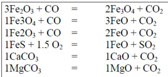
**Figure 7. Chemical reactions resulting in process emissions (EC, 2007, p. 58).**
