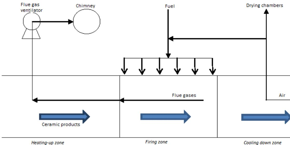
**Figure 12. Three phases of the firing process in a tunnel kiln: heating-up, firing and cooling down zone. Source: captured and translated from (Ecosys, 2014, p. 36).**
