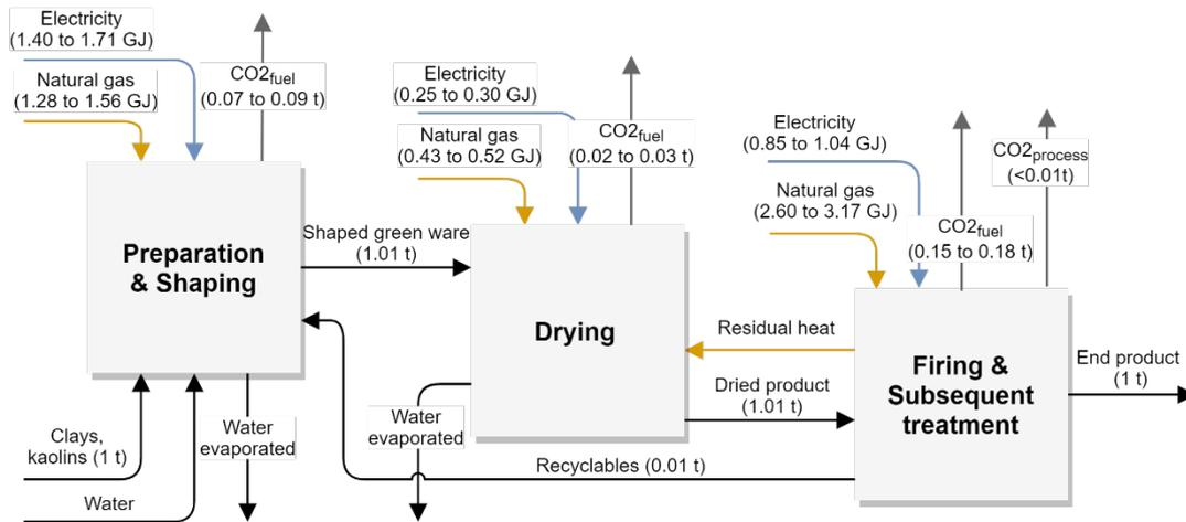
**Figure 17. Flow diagram of the manufacturing process of floor tiles, including material, energy and CO<sub>2</sub> emissions flows.**
