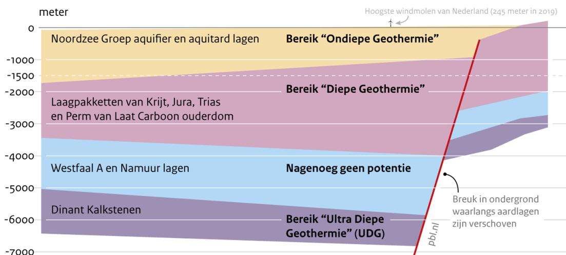
**Figure 26. Different earth layers that specify the type of geothermal heat. Source: (Lensink, 2020)**
