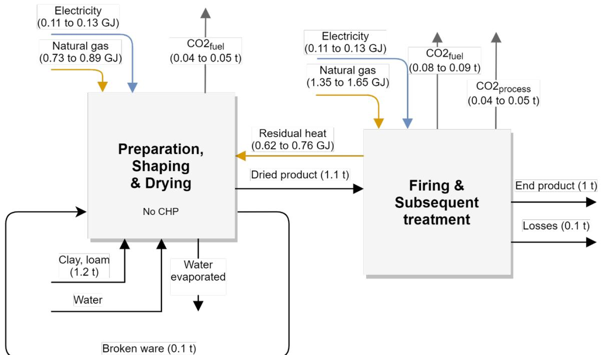
**Figure 14. Flow diagram of the manufacturing process of bricks and roof tiles, including material, energy and CO<sub>2</sub> emissions flows. Applicable to plants without gas-fired CHP, steam boilers for drying, or other alternative drying methods.**
