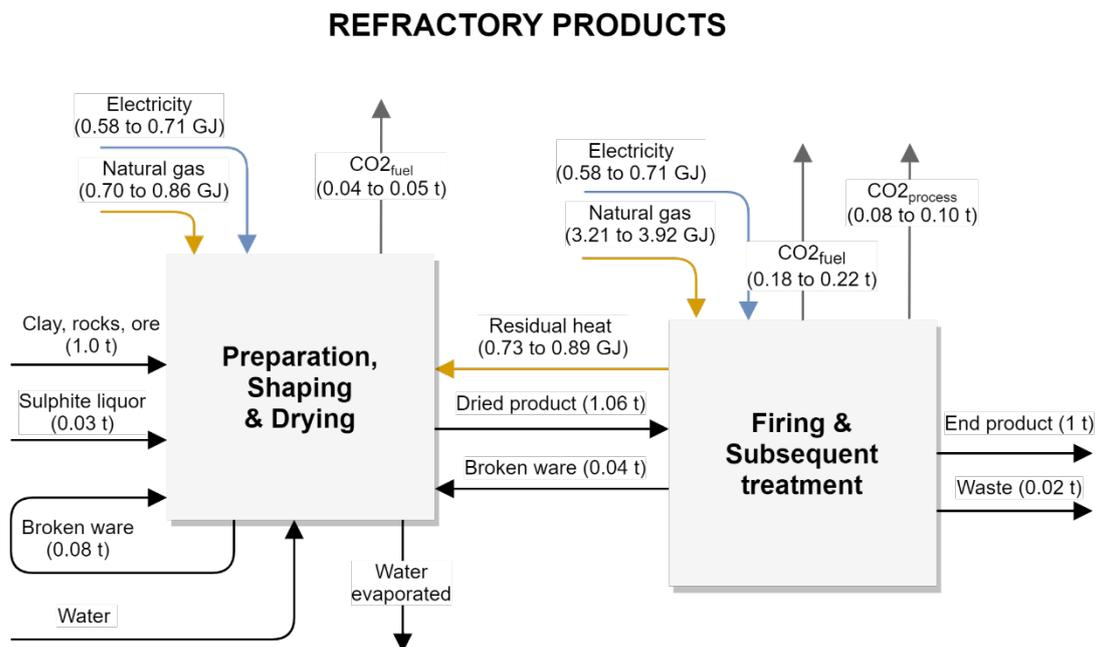
**Figure 19. Material, energy and CO<sub>2</sub> emissions flow diagram of refractory products. Material amounts are taken from the BREF example of production of periclase chromite bricks (EC, 2007, p. 112).**
