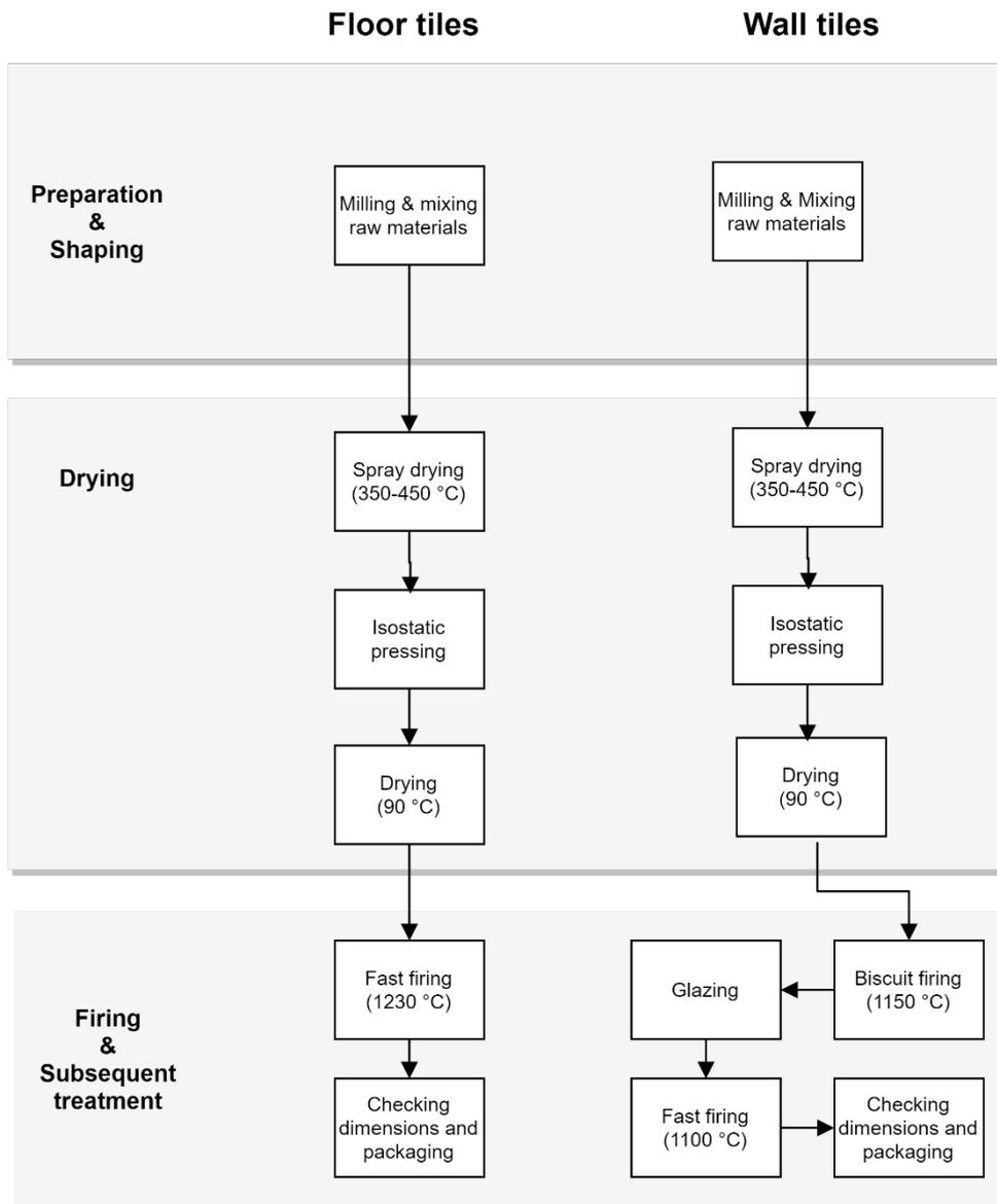
**Figure 15. Production processes wall and floor tiles**
