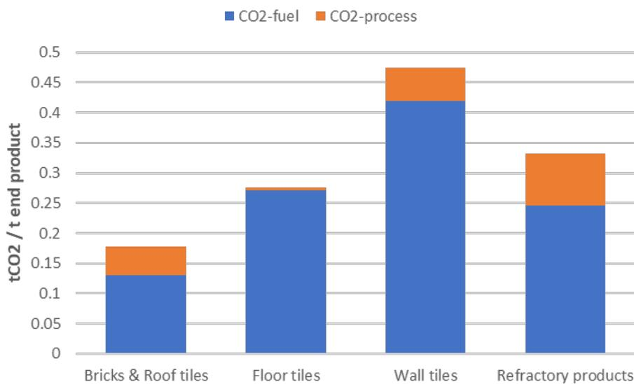
**Figure 8. CO<sub>2</sub> emissions per tonne of end product per product type. Blue part of the bar are emissions from burning fuels and orange part are the process emissions. This graph is based on the analysis in this chapter and Appendix A.**
