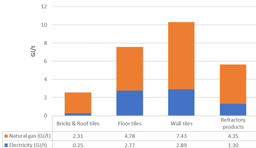
**Figure 4. Energy input per fuel per tonne product of each category, based on the analysis in the chapter and Appendix A.**
