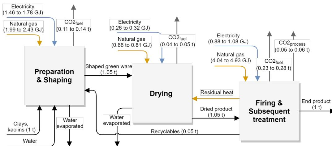
**Figure 18. Flow diagram of the manufacturing process of wall tiles, including material, energy and CO<sub>2</sub> emissions flows.**
