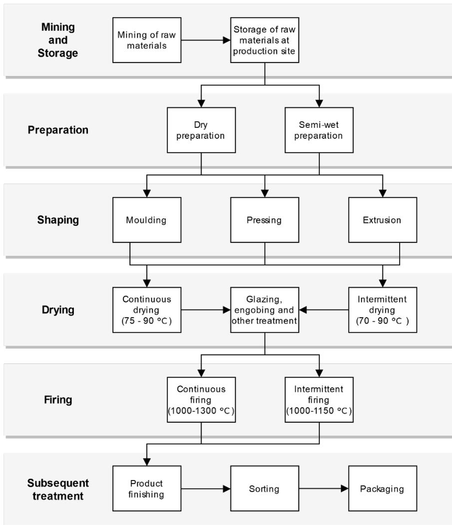
**Figure 10. Production processes bricks and roof tile manufacturers.**
