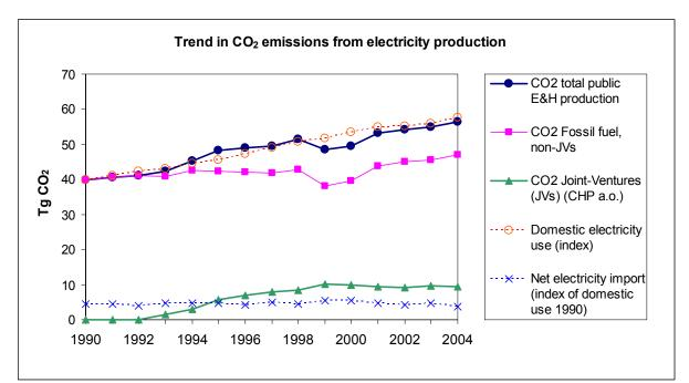
Figure 3.2 Trends in CO<sub>2</sub> emissions from public electric power generation (including public heat production).
