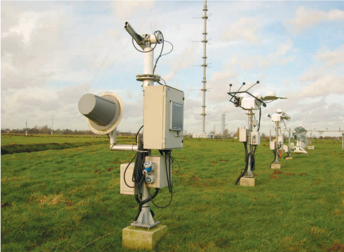
Figure 2.3 A Cimel sun photometer set-up as an AERONET station, including a solar panel for electrical power and a transmitter for relay of data to AERONET headquarters at NASA-GSFC. (Photo: Ed Worrell/KNMI).
