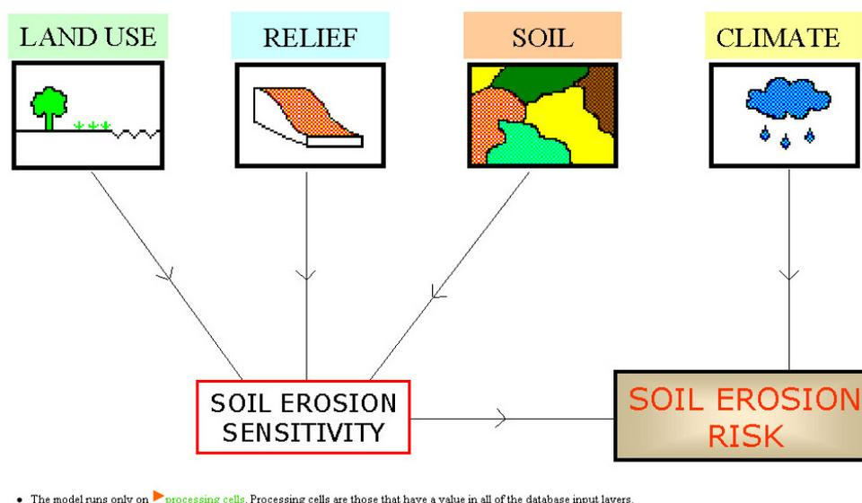
Figure 6.23. Concept of INRA method
