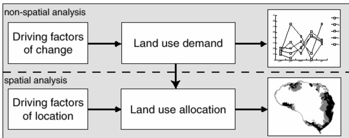
Figure 4.9: Overview of the modeling procedure.
