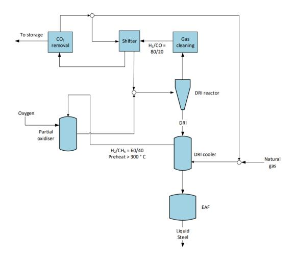
Figure 14. Basic schematic of natural gas-based ULCORED
