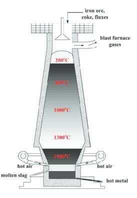
Figure 3. Schematic diagram of the blast furnace process
