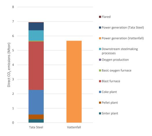
Figure 8. Calculated annual direct CO<sub>2</sub> emission distribution of steelmaking units and power generation plants
