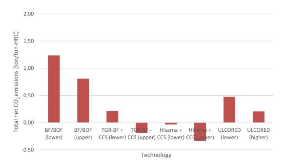
Figure 32. Comparison of CO<sub>2</sub> emission estimates with charcoal substitution in the most feasible steelmaking technologies
