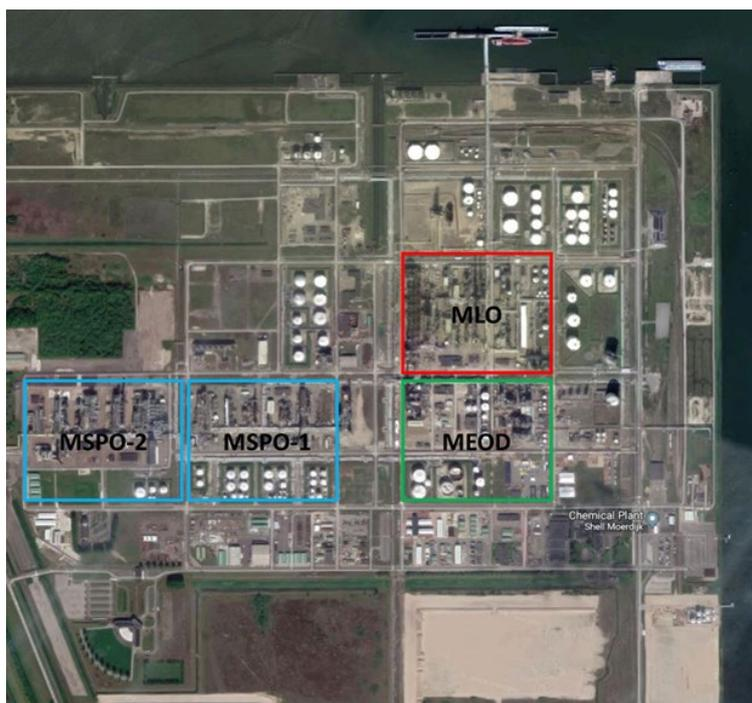
**Figure 1.3 Shell Moerdijk site with main activities/plants indicated (MLO = Moerdijk Lower Olefins, MSPO = Moerdijk Styrene monomer and Propylene Oxide, MEOD = Moerdijk Ethylene Oxide and Derivatives)**
