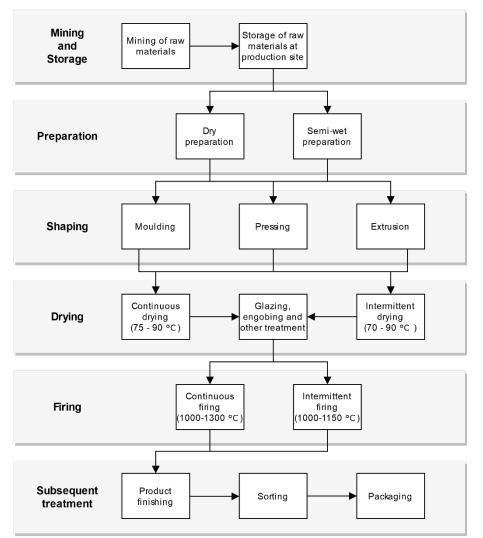
Figure 10. Production processes bricks and roof tile manufacturers.
