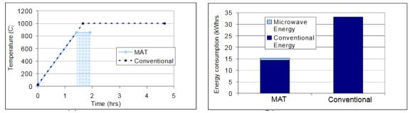
Figure 25. On the left the temperature and duration of the firing process and on the right the total energy consumption. Source: (Shulman, 2007).
