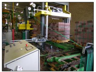
Figure 13. Packaging machine of bricks (KNB, 2020).
