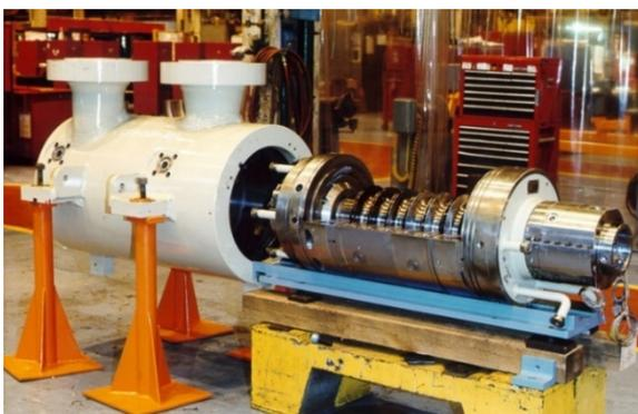
**Figure 17. Assembly of a centrifugal compressor (Turbomachinery International, 2016)**
