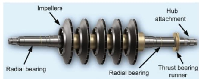
**Figure 16. Components of a typical rotating assembly in a centrifugal compressor (Brun et al., 2018)**
